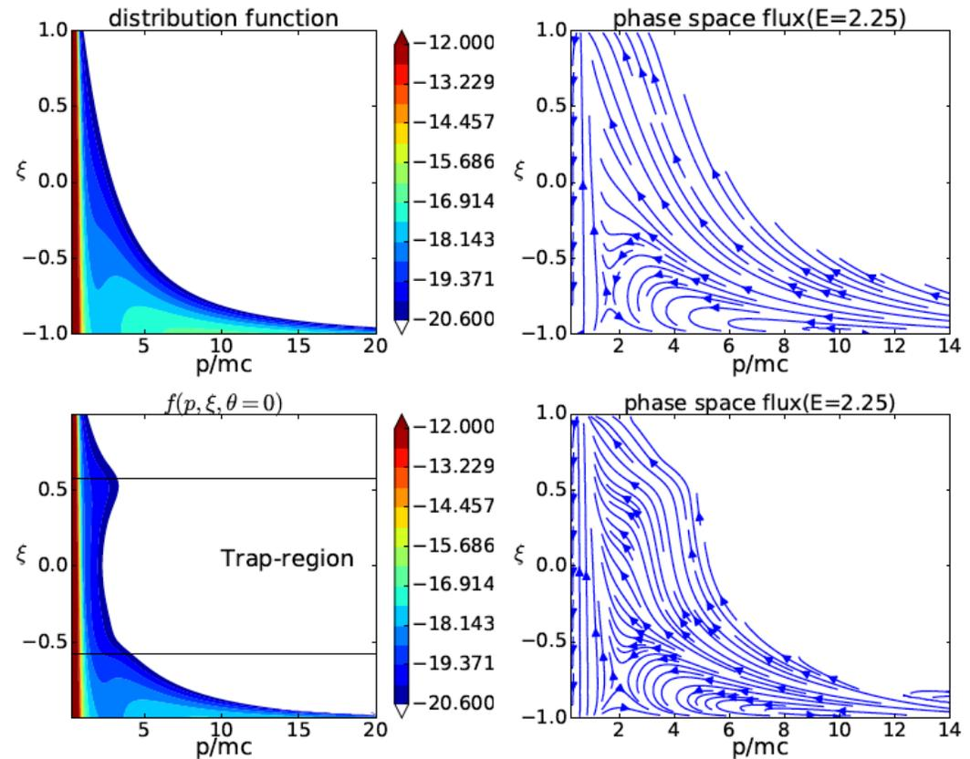
FIG. 1. TOP:  $f(p, \xi)$  and phase-space flow in slab geometry with  $E = 2.25E_c, \alpha = 0.2, Z = 1$ ; BOTTOM:  $f(p, \xi, \theta = 0)$  and phase-space flow in tokamak geometry with  $E = 2.25, \alpha = 0.2, Z = 1, r/R_0 = 0.2$
