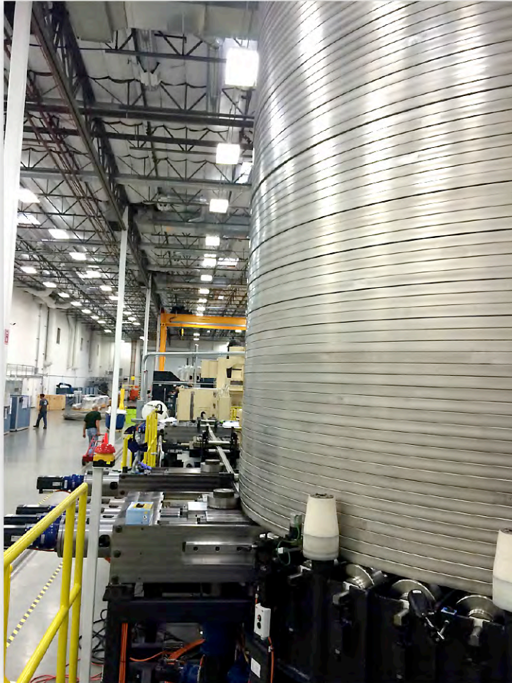
Conductor routed from the de-spooler of the winding.
