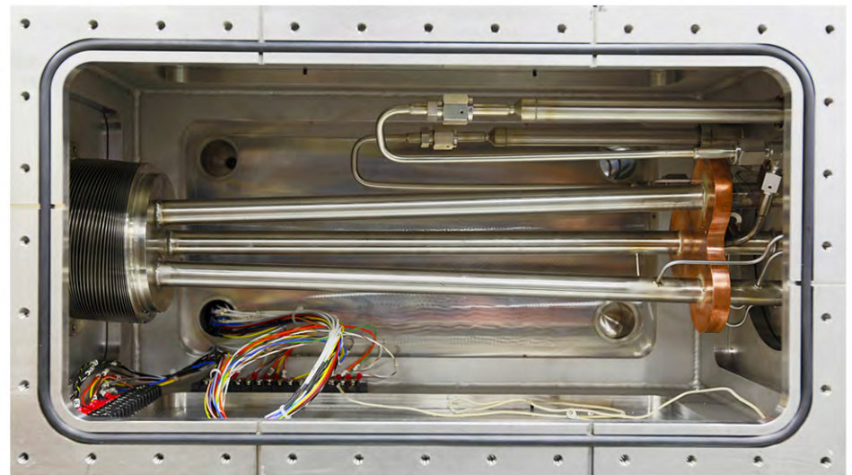
3-barrel unit prototype for disruption mitigation
