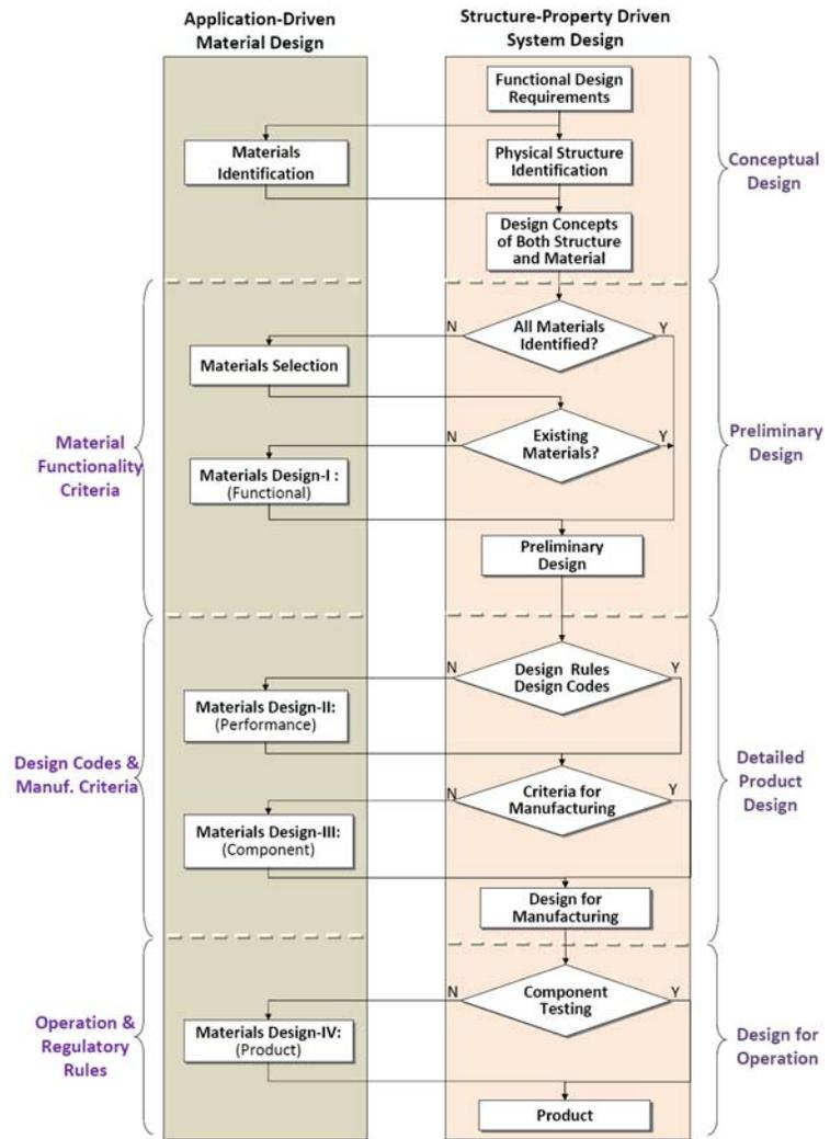
Fig. 1: Idealized process flow showing the integration of material development and design [S. Sharafat, ICFRM-13].
