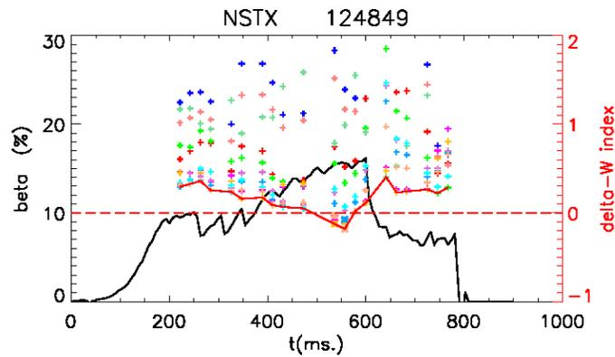
Figure 1. Evolution of  $\beta$  and the minimum of the potential energy, based on a pre-determined set of eigenvectors. The crosses, represent  $\delta W(\xi_i)$ , for each time slice. The red line tracks the minimum. Note that it steadily decreases reaching its minimum, shortly before the beta collapsed.
