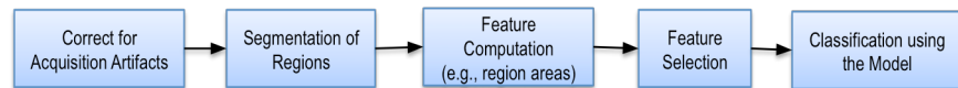
Figure 2. Workflow for analysis of 2D image data as one of ensemble of workflows for instability prediction during experiment run.
