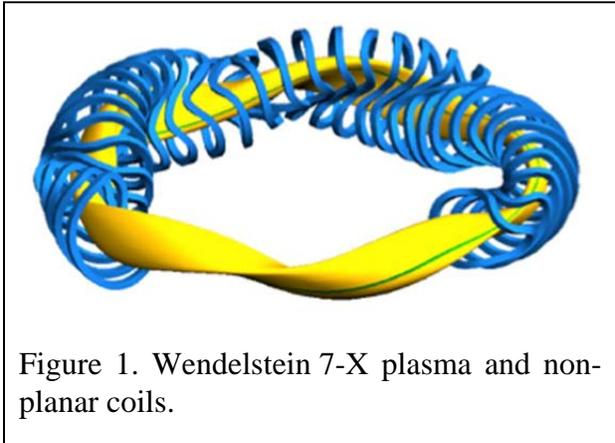
Figure 1. Wendelstein 7-X plasma and non-planar coils.
