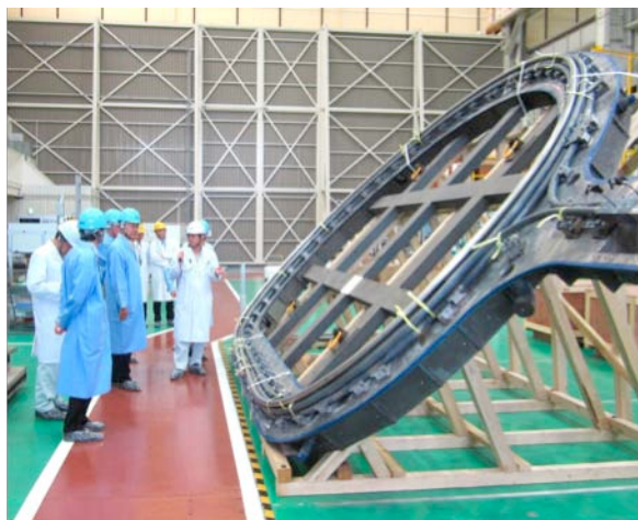
Delegation viewing a mockup of a section of TF coil case at Toshiba, Keihin Product Operations, Yokohama, Japan (photo courtesy of ITER Organization)
